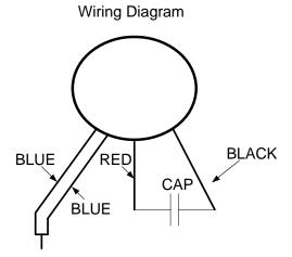
Capacitors are non-polarized and must always be connected between the red and black leads. Always connect the (2) coil blue leads together. Connect the power supply to the blue leads and red lead to produce clockwise (CW) rotation viewing shaft end. Connect the power supply to the blue leads and black lead to produce counter-clockwise (CCW) rotation viewing shaft end. Optional Wiring Diagram with Switch
