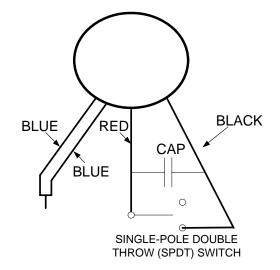
Capacitors are non-polarized and must always be connected between the red and black leads. Always connect the (2) coil blue leads together. Connect the power supply to the blue leads and red lead to produce clockwise (CW) rotation viewing shaft end. Connect the power supply to the blue leads and black lead to produce counter-clockwise (CCW) rotation viewing shaft end.
