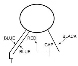
Capacitors are non-polarized and must always be connected between the red and black leads. Always connect the (2) coil blue leads together. Connect the power supply to the blue leads and red lead to produce clockwise (CW) rotation viewing shaft end. Connect the power supply to the blue leads and black lead to produce counter-clockwise (CCW) rotation viewing shaft end.
